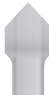
CRIMPED SPEAR TOP DETAIL
