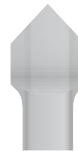
CRIMPED SPEAR TOP DETAIL
